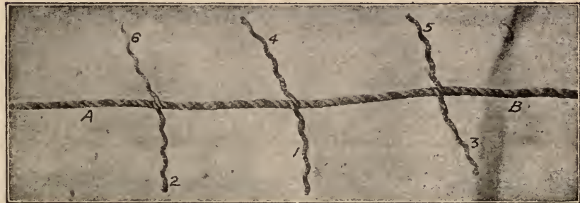
Fig. 10. Ready to Tie the Knots in the Long Splice. Ends 1, 2 and 3 Are from Rope A. Ends 4, 5 and 6 Are from Rope B
