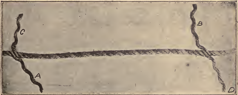
Fig. 5. The New Strand Has Been Laid In Ready to be Secured at the Ends.
