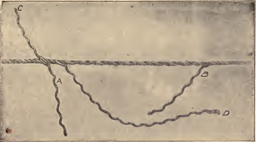
Fig. 4. In Laying In the New Strand the Original Twist and Tension Must Be Maintained
